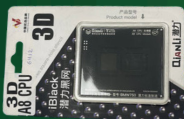
REBALLING STENCIL 3D Black CPU A8
