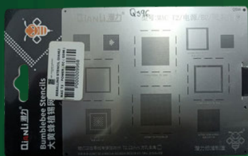
REBALLING STENCIL Power- EC QS96
